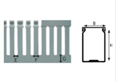
Iboco T1-EF range is ideal for small sized wires commonly employed in electric control panels. It has restricted slot opening and its strong and robust due to its thick base and side construction. Perfect solidity is also guaranteed in cantilevered applications. Made of material with more than 3000NPa modules of elasticity, it allows for repeated opening and closing of the duct fingers during wiring operations even at low temperature, without breaking.
